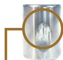
ENGINE OIL EXTREME WEAR at 4 Loads
